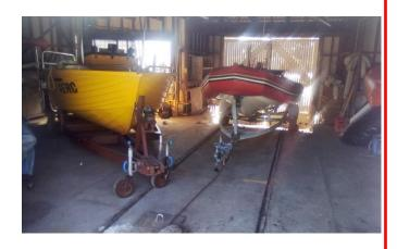
**Launching Red Rib:** Check bungs and motor is tilted fully up.
